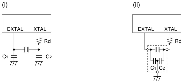
Fig. 13. SPC700 Series recommended oscillation circuit
