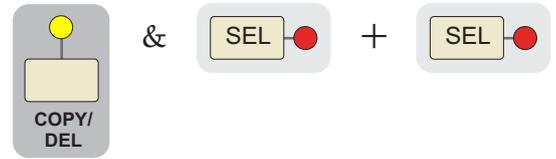
Note that Copy/Swap is only allowed between similar modules; the unit will not allow you to swap settings between an EQ module and a Dynamics module for instance!
