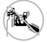
Do not modify or alter an aerial work platform without prior written permission from the manufacturer. Mounting attachments for holding tools or other materials onto the platform, toeboards or guard rail system can increase the weight in the platform and the surface area of the platform or the load.
