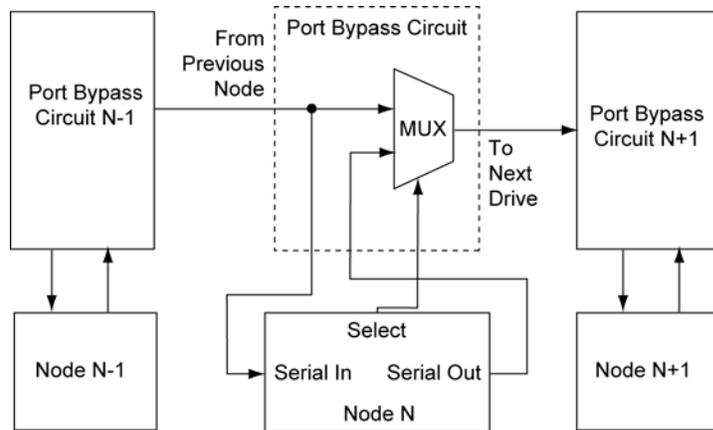
**Figure 6.** Typical Backplane Bypass Circuit
