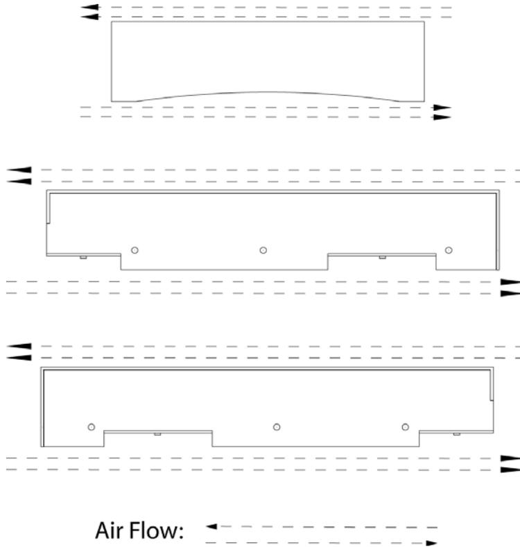
**Figure 10.** *Suggested Air Flow Patterns for Cooling*
