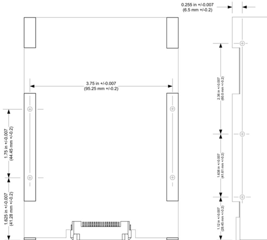
**Figure 11.** Exterior Mounting Specifications
