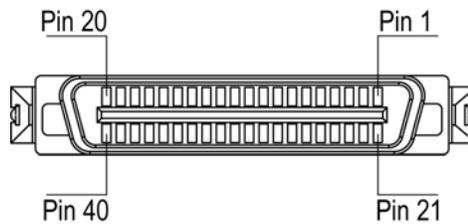
**Figure 2.** SCA-2 Interface Connector
