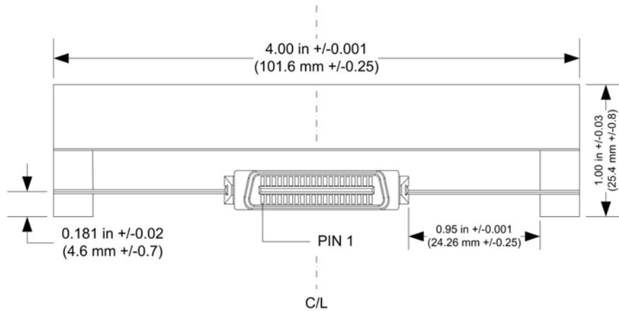
**Figure 3.** Relative SCA-2 Connector Location
