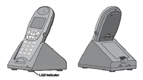
The Dual Charger is designed to charge the Battery Pack in the handset while it remains operational and also charge an additional Battery Pack in the rear charging bay. The handset has charging priority when both slots are occupied.
