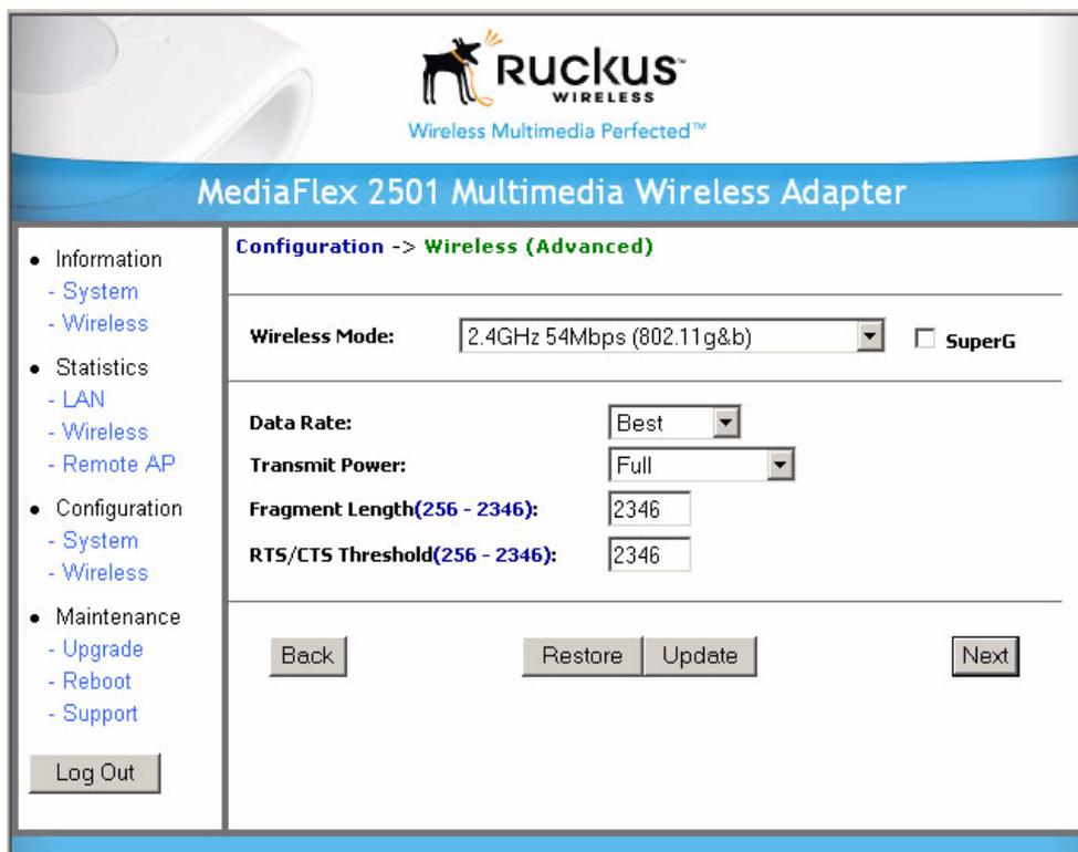
**Figure 7**—Advanced Wireless Configuration
