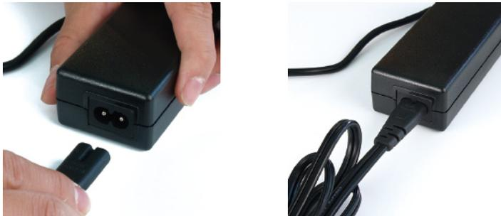
3. Plug the power adapter to your ATA/ATAPI device. Please check a to d as below.
