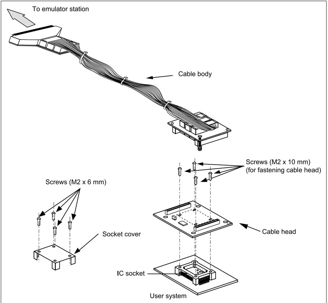
**Figure 1 HS2655ECH61H User System Interface Cable**
