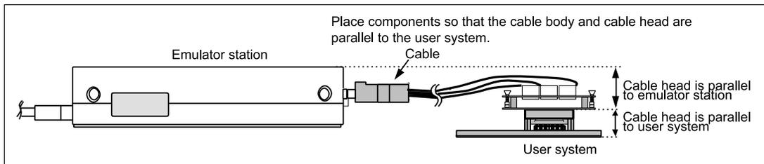
**Figure 11 User System Interface Cable Location Example**
