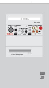
Select the drive bay you wish to mount the GCi404 into. Remember that you will have cords hanging down from the unit, so below a CD Rom drive is recommended. Remove the drive bay cover and gain access to the inside of vour computer.
