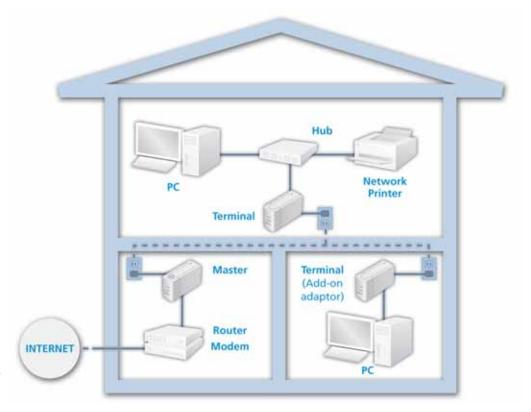
The Ricoh HD-PLC Ethernet Adaptor uses the existing electrical wiring system in your building to allow connected users to share data, networked peripherals, and to access the Internet through any AC power outlet.
