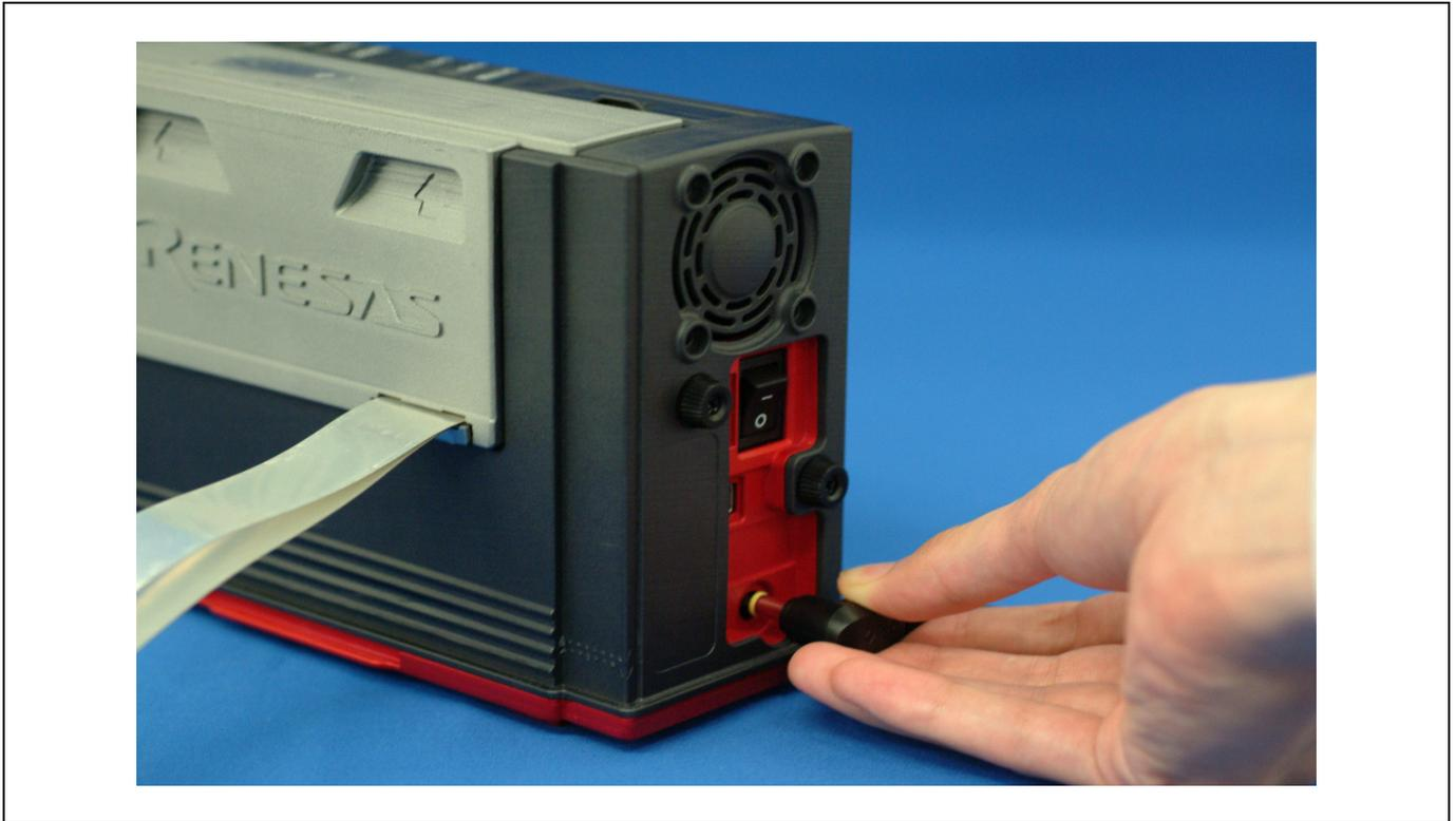
Figure 2.5 Connecting the emulator power supply
