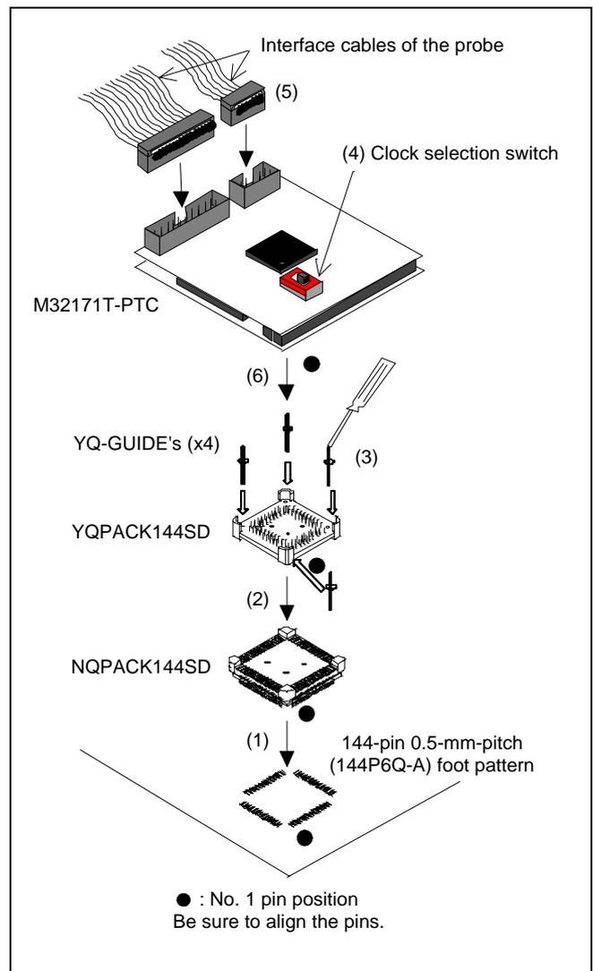
Figure 3 Attaching procedure of the M32171T-PTC
