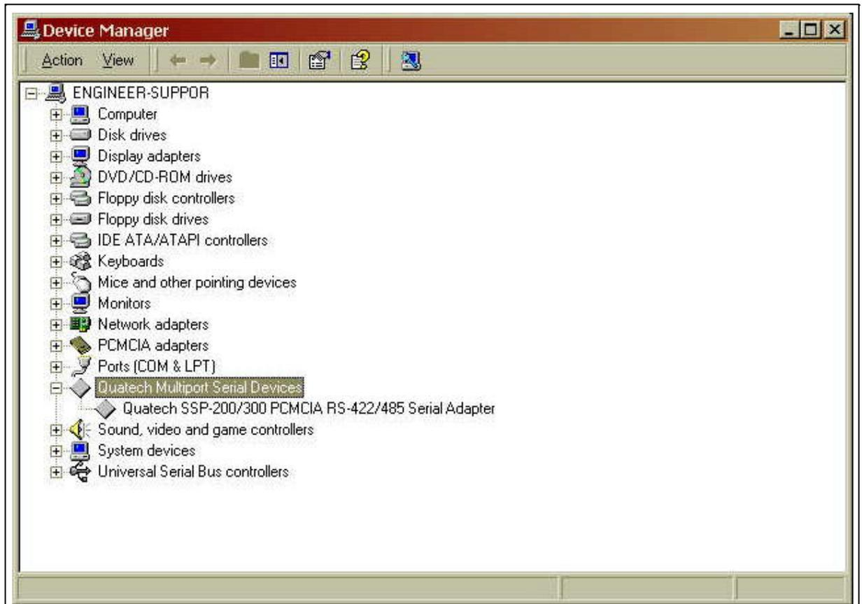
3. The SSP-200/300 “parent device” belongs to this hardware class. The device name for the SSP-200/300 is **Quatech SSP-200/300 PCMCIA RS-422/RS-485 Serial Adapter**.
