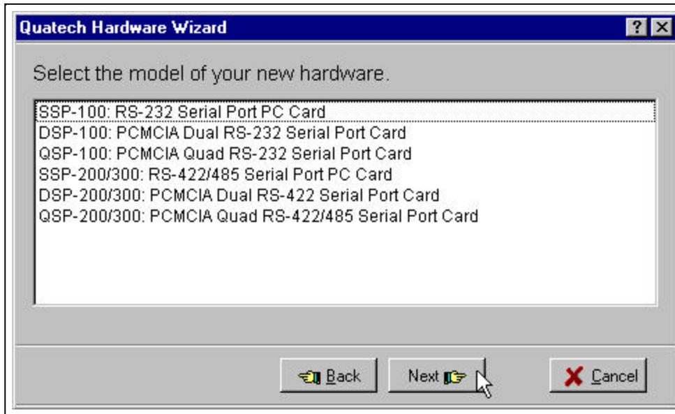
4. Complete the final steps of the installation, shut down Windows NT and then insert the PCMCIA Card and re-boot the computer.
