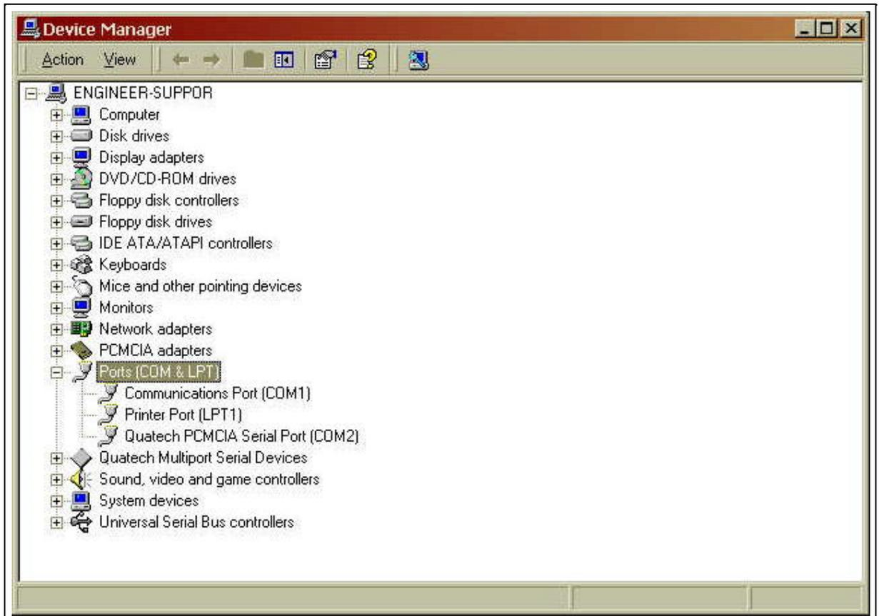
6. Use the COM Port device names (COM5, COM6, etc.) to access any of the particular serial ports on the SSP-200/300. This name is required by a Windows **2000** application when accessing a particular port.
