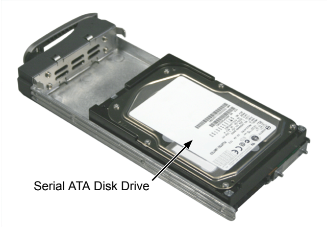
Figure 13. SATA Disk Drives mount at the front of the carrier
