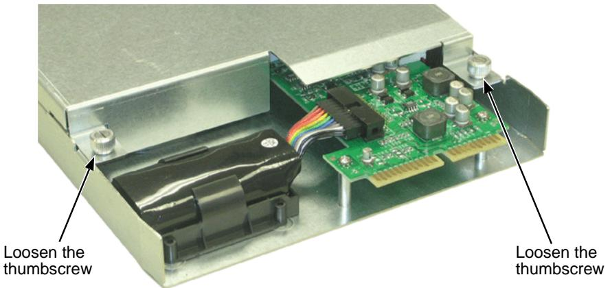
5. Loosen the thumbscrews (above). Retainers keep the thumbscrews in place.
