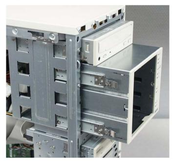
5. If your PC chassis uses slide brackets (above), attach two slides to each side of the SuperSwap enclosure. Otherwise, continue with Step 6.
