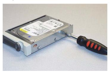
2. Install and tighten the four mounting screws through the *sides* of the drive carrier (above).
