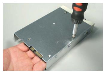
2. Carefully turn the drive carrier over and support the disk drive. Install the four countersink screws through the holes in the bottom of the drive carrier, to attach the disk drive. Gently tighten the screws.
