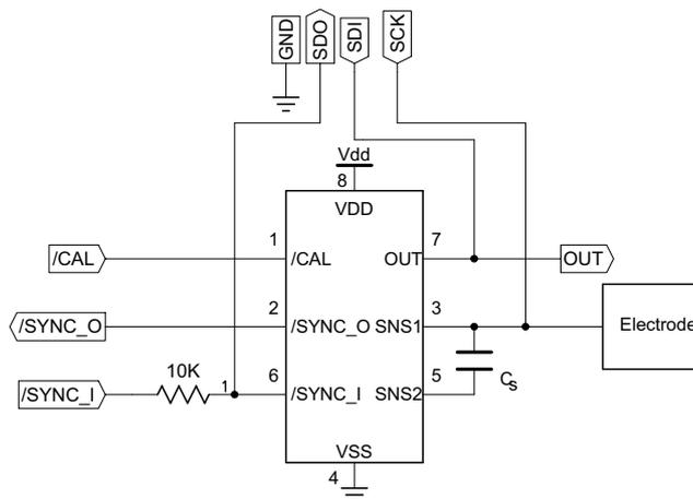
**Figure 5 - QT320 Clone Connections**
