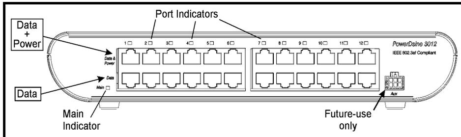
Figure 2-1: Power over LAN Midspan, Front View (PD-3012)
