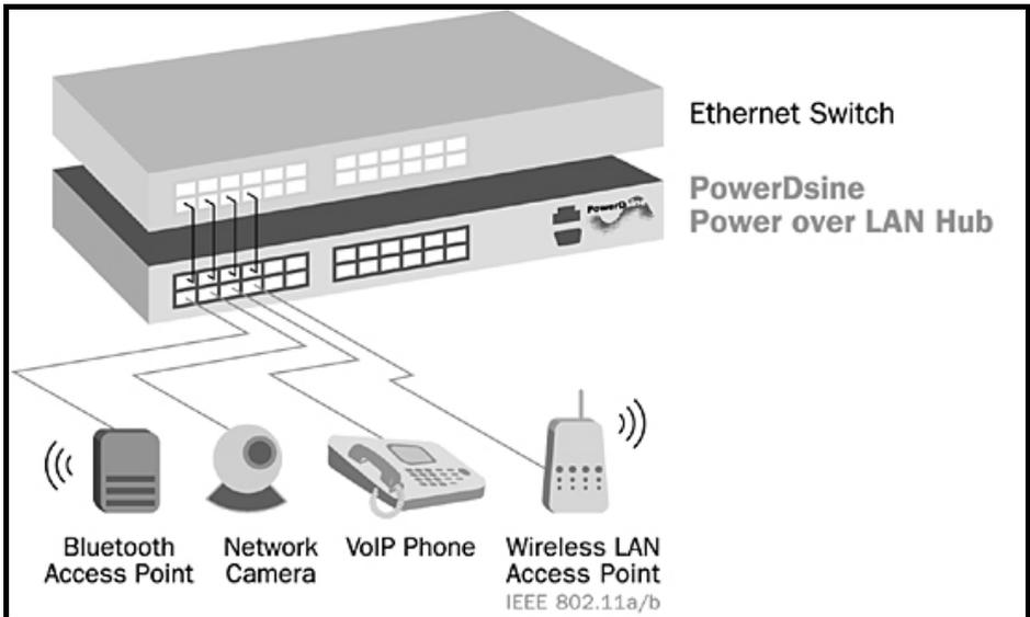
Figure 3-1: Typical Installation
