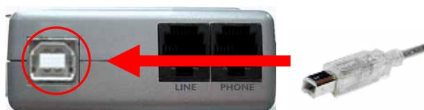
The other end of the USB cable must be connected to a USB port on your computer as shown below, or to an AC Powered USB hub.
