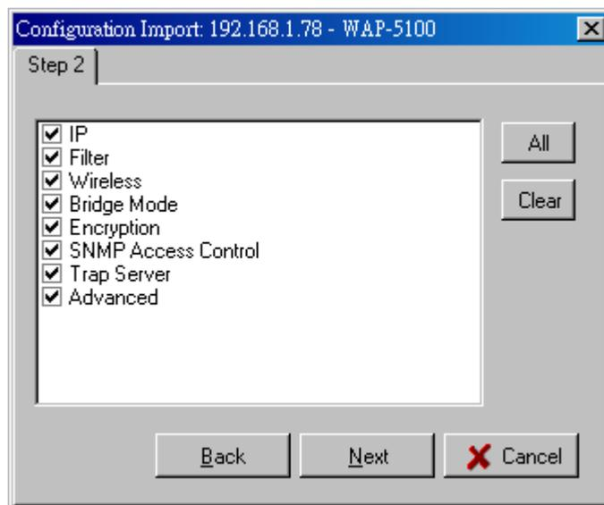
The configuration profile does not contain the security key settings. The attributes of security keys are externally write-only and cannot be saved into the configuration file. If you select **Encryption** session to be imported, it will display the **Encryption** window before Step 3 screen and ask you to enter the security key settings manually.
