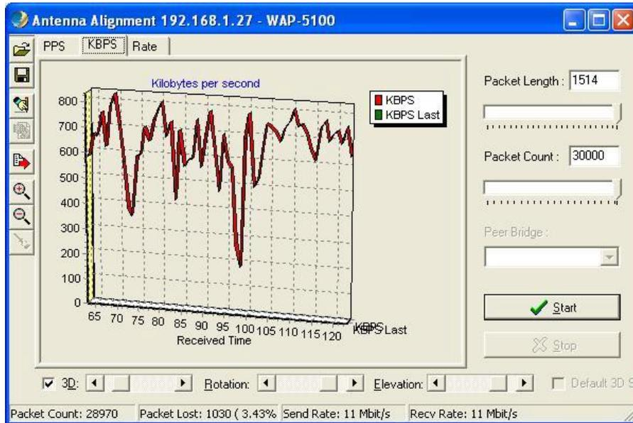
During the antenna alignment test, the bridge might receive interference owing to some unexpected reason. Under this circumstance, the wireless communication data rate will automatically fall back. The numbers of packets sent or received at different data rates can be viewed as shown below .
