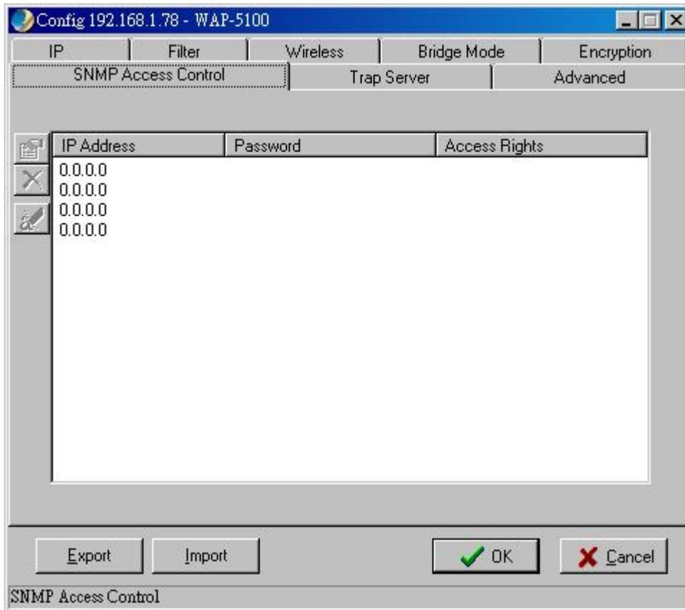
When you select **SNMP Access Control**, the system will display four blank fields for setting (maximum of 4 SNMP devices can be set). Right-click on a blank in the list and click **Edit Address**. The **New/Edit Address** dialog box will appear. Type in the IP address and set the password for the SNMP device. There are two levels of access rights can be assigned:
