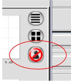
A window would appear on the screen to prompt user for the SNMP version to use and its corresponding community or passwords. Click the **Block User** button once completed the step, the selected client will be removed from the active client table, and added into the MAC Access Table.
