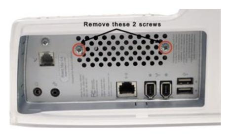
Unscrew these two screws from the rear port panel on your system. This will release the fan from behind the heatsink and allow you to unhook the rear heatsink clips in the next step. You will not be reinstalling this fan.
