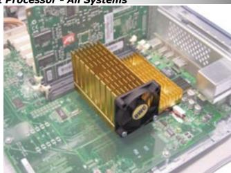
Installation of the processor daughtercard is the same on all systems, simply align the 3 screw holes in the card and gently place over the logic board. Gently but firmly press straight down on the two rearmost screwholes until you feel the card "click" into place. Insert the included screwdriver and tighten the encapsulated 3 Phillips screws into the 3 screw holes.
