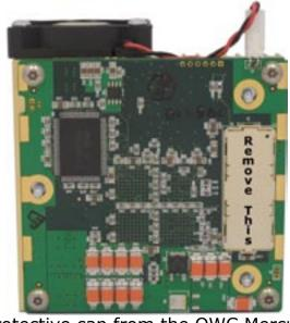
Remove the protective cap from the OWC Mercury Extreme G4 processor upgrade. The cap is located on the bottom of the card, between the screw holes. Place the cap onto the processor card you just removed.
