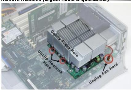
Remove the heatsink from your logic board. Use the needle nose pliers to unhook the clips from the processor card. If your system includes a processor fan or cover, unplug it and then remove by unclipping it and pulling straight up and out. You will not be reinstalling this heatsink, fan or shroud.
