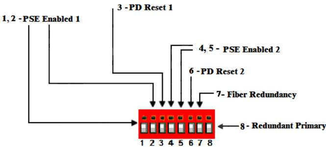
**Note:** All switch changes take effect immediately. Switch changes will cycle power to the PD only if the PD Reset switch is set to On or you make changes to the PSE Power switches.
