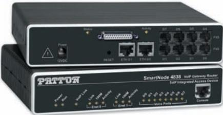
The SmartNode™ 4830 Series IADs let you deliver voice-over-IP over virtually any WAN access link type. The series offers models with combinations of 2 to 8 analog FXS phone ports and 2 or 4 FXO ports. Each model has two Ethernet ports and an integrated WAN access modem—choose from X.21, V.35, T1, E1, G.SHDSL or ADSL2+ to match the given access link with greatest flexibility. Quality
