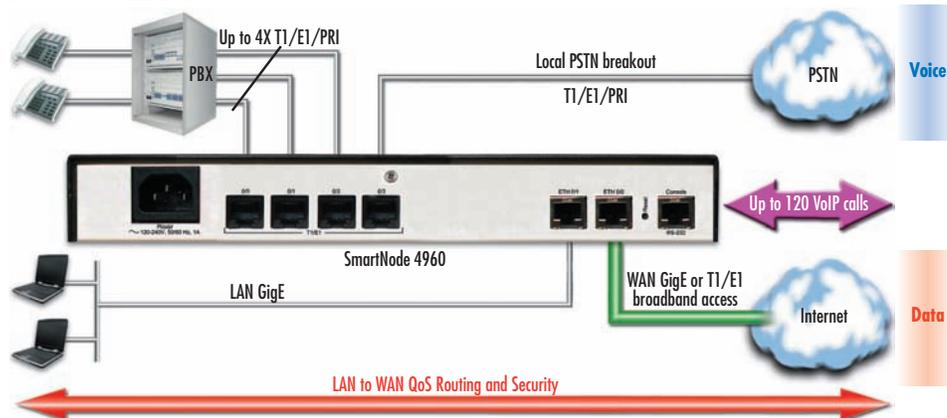
**IpChannel Bank Multi-Port FXS & FXO Gateway Router**
