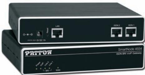
The SmartNode™ 4554 ISDN BRI PSTN Gateway converts up to four simultaneous phone or T.38 fax calls from SIP or H.323 to BRI ISDN. It is a compact reliable stand-alone VoIP gateway for IP-based voice systems that delivers ISDN performance and quality.
