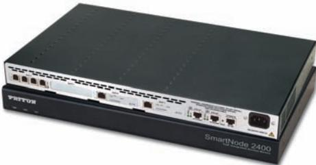
The SmartNode 2400 Series provides a high density, seamless link between the circuit-switched telephone network and Voice-over-IP. Ideal for multi-service carrier and corporate PSTN access, the SmartNode 2400 Series takes 120 calls from voice-to-packet. With dual 10/100 Ethernet ports and four voice interface slots, the SmartNode 2400 connects to any switch, PBX, or data network.
