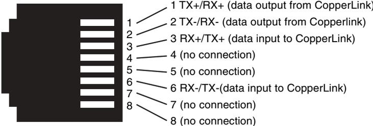
Figure 7. CopperLink Ethernet Extender 10/100Base-T RJ-45 Connector Pinout.
