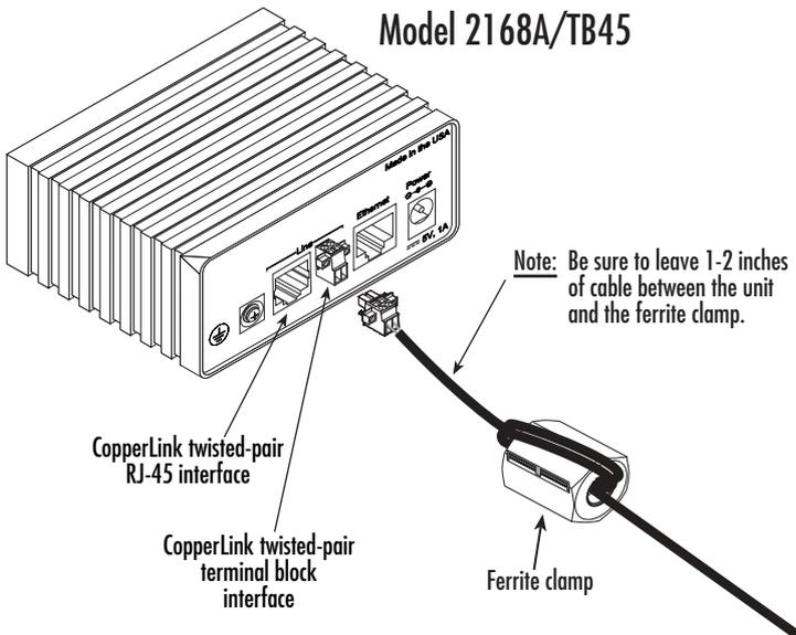
**Figure 6.** Connecting the ferrite clamp for 2168A/TB45 models
