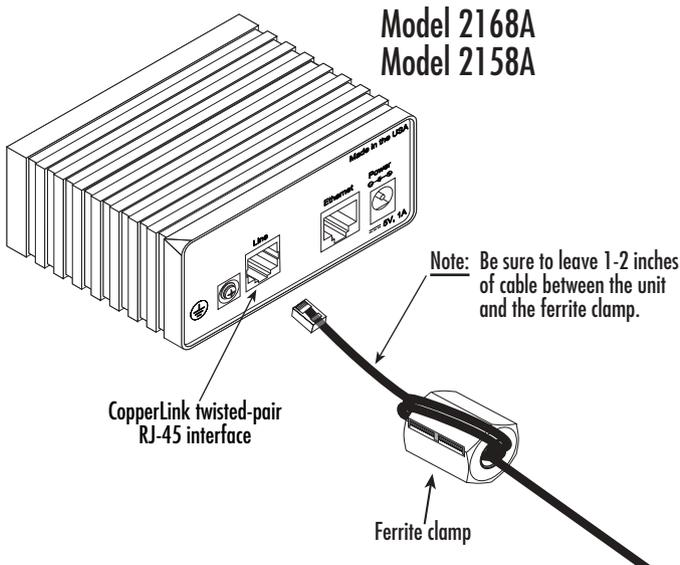
Figure 5. Connecting the ferrite clamp for 2168A/2158A models
