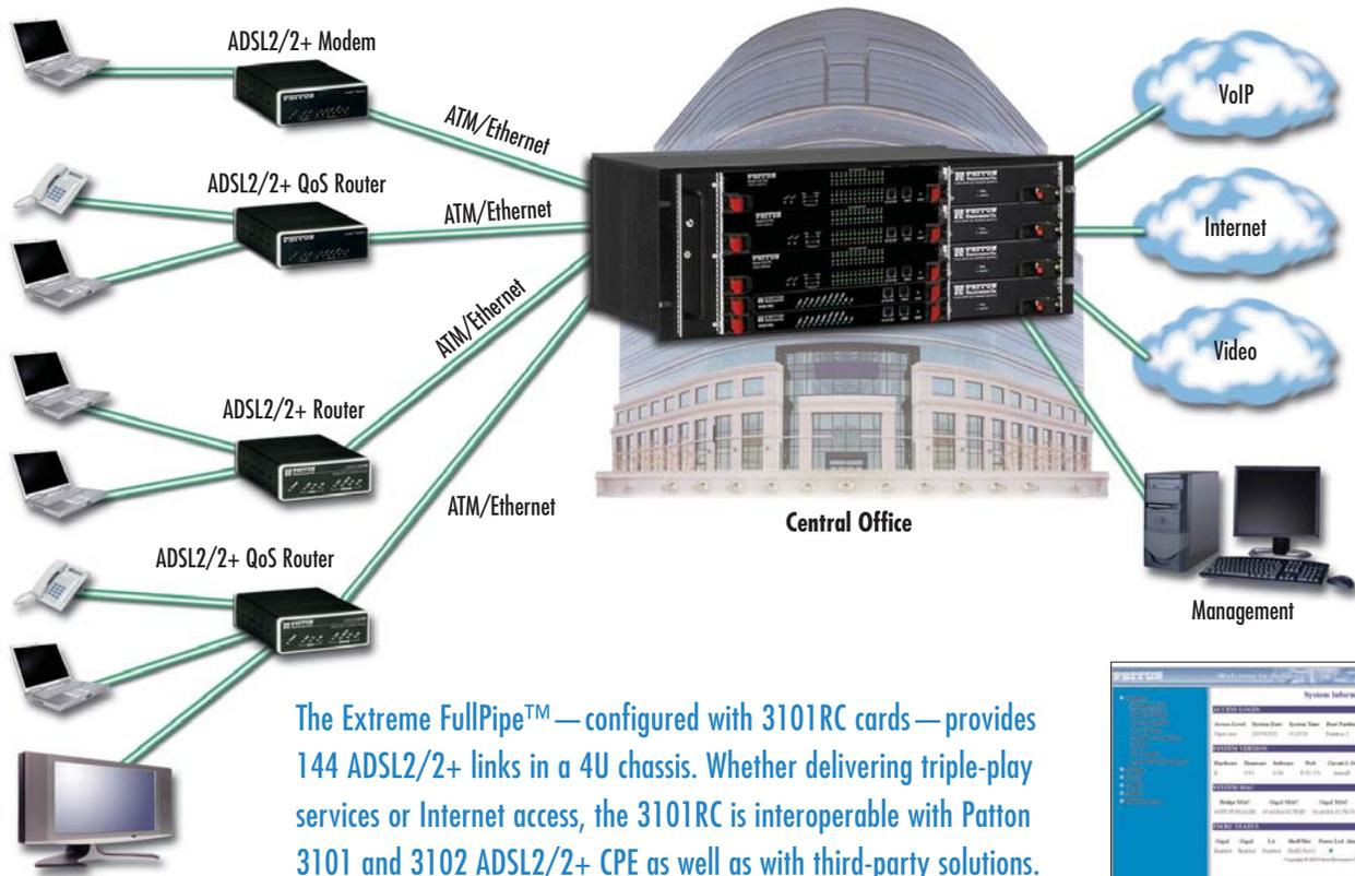
The Extreme FullPipe™—configured with 3101RC cards—provides 144 ADSL2/2+ links in a 4U chassis. Whether delivering triple-play services or Internet access, the 3101RC is interoperable with Patton 3101 and 3102 ADSL2/2+ CPE as well as with third-party solutions.
