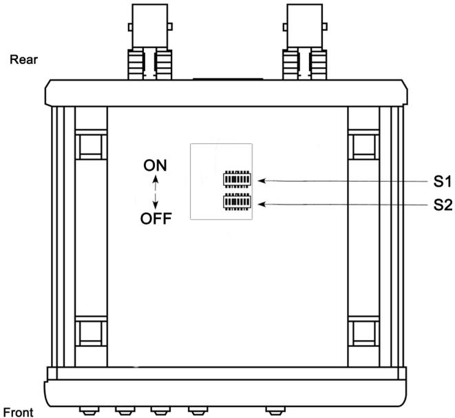
*Figure 1.* Underside of Model 2707, Showing Location of DIP Switches
