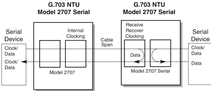
**Figure 7.** Local Loopback for a Network Termination Application
