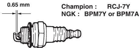
Clean the electrodes with a wire brush and reset the gap to 0.65 mm as necessary.
