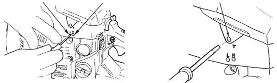
The carburetor on your unit has been factory adjusted, but may require fine tuning due to a change in operating conditions.
