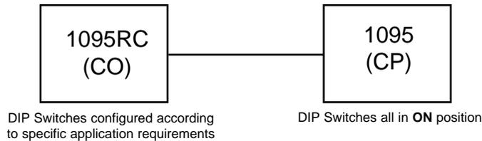
Figure 3. Typical NetLink Plug-and-Play Application
