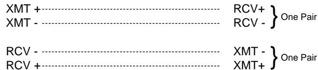
5. When you finish connecting the wires to the terminal block, the assembly should resemble the diagram Figure 6 below.
