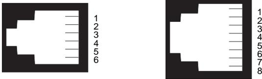
AT&T standard modular pin assignments
