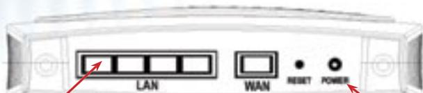
Plug your computer's Ethernet cable into Port 1. The remaining ports can be used with other computers in a hard-wired router fashion.
