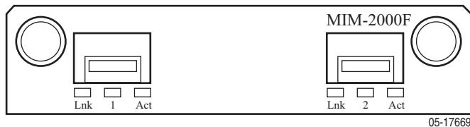
All MIMs are hot-swappable, although removal of a MIM disengages the upstream network connection for the DSLAM.
