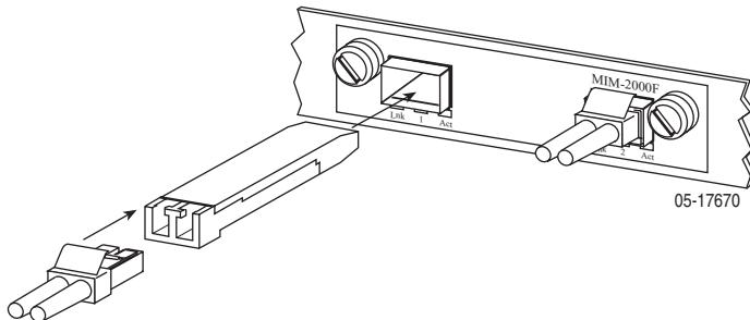
To install SFP transceivers in the MIM-2000F:
