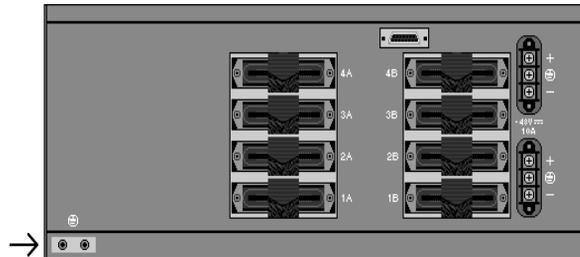
Ground Connection for 2-Hole Terminal Lug
