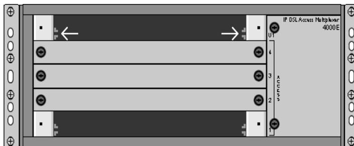
3. Slide the Management Module Firmly into the Chassis. Tighten the fastening screws on the management module faceplate.
