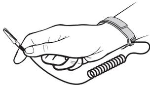
This product is designed to protect sensitive components from damage due to electrostatic discharge (ESD) during normal operation. When performing installation procedures, however, take proper static control precautions to prevent damage to equipment. If you are not sure of the proper static control precautions, contact your nearest sales or service representative.
