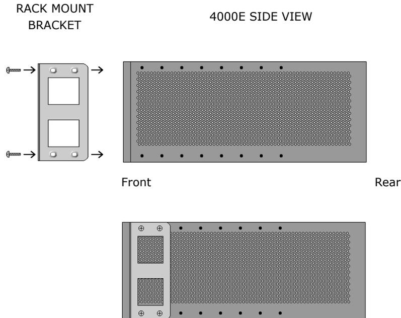
Mount the chassis onto the rack and secure the rack mount brackets to the sides of the rack using one of the two provided sets of eight [8] rack screws (whichever size fits the rack being utilized).
