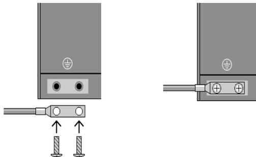
2. Connect the Ground Wire to a Frame Ground. Ground wire connection can vary from location to location, although typically all equipment in a Central Office is grounded to a common copper bus.
