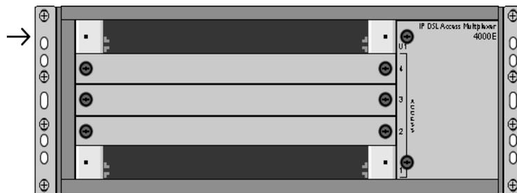
2. Align the management module with the slot module guides. With the management module printed circuit board (PCB) facing up and the management module model name on the right side of the module faceplate (facing towards you), align the left and right edges of the PCB with the U1 slot module guides on the 4000E.
