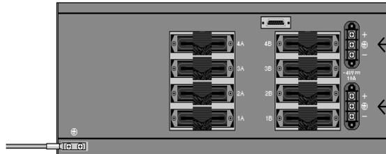
4. Select a terminal block. Using a Phillips Screwdriver, remove the upper screw from the chosen terminal block (labeled "+" on the chassis). Slide the ring terminal of your positive power lead around the shaft of the screw and insert the screw into the same "+" terminal from which it was removed.
