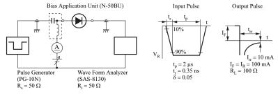
\*2: Mounted on an alumina PC board (board: 20 mm  $\times$  50 mm  $\times$  0.8 t, soldering land: 2.0 mm  $\times$  2.0 mm + 20 mm  $\times$  0.8 mm)
