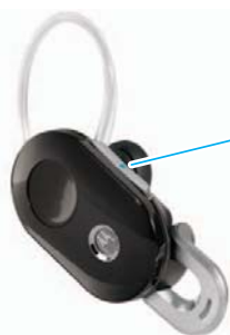
Indicator Light (steadily blue for pairing mode)
