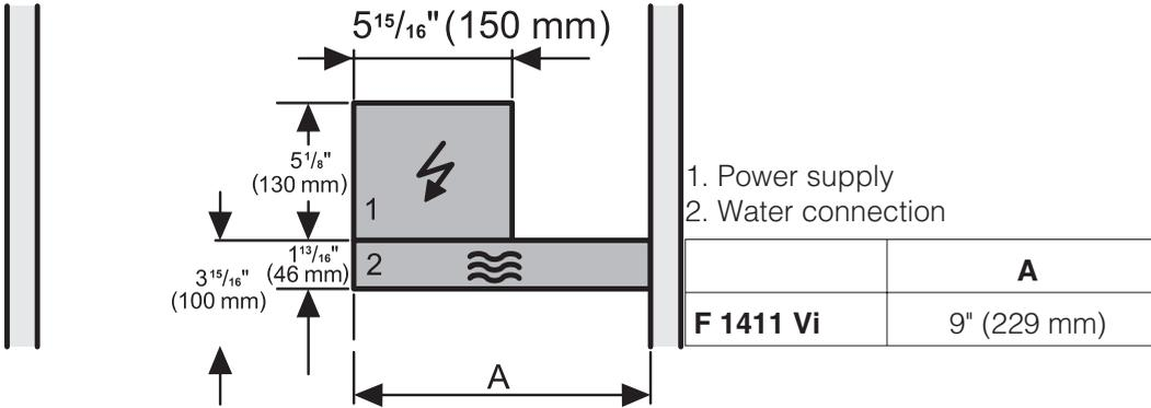
Install a pressure limiting device and water hammer arrester for inlet water pressures exceeding 80 psi. (Refer to Uniform Plumbing Code, Sections 608.2 and 609.10) Never install or operate where inlet water pressure may exceed 120 psi.
