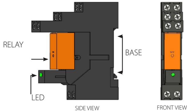
The FLEXware Relay Assembly will activate a two-wire start generator when wired to the AUX output of either an OutBack FX Inverter/Charger or an OutBack Charge Controller. The assembly consists of an LED module and a relay inserted (in one orientation) into a base. The base is mounted onto the DIN rail of any OutBack AC industrial control panel.
