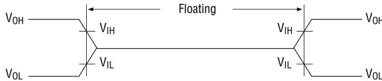
\* The port 0 floating interval is measured from the time the port 0 pin voltage drops below  $V_{IH}$  after sinking to GND at 2.4 mA when switching to floating status from a "1" output, and from the time the port 0 pin voltage exceeds  $V_{IL}$  after connecting to a 400  $\mu$ A source when switching to floating status from a "0" output.
