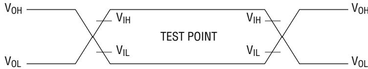
\* The input signals in AC test mode are either  $V_{OH}$  (logic "1") or  $V_{OL}$  (logic "0") input signals where logic "1" corresponds to a CPU output signal waveform measuring point in excess of  $V_{IH}$ , and logic "0" to a point below  $V_{IL}$ .
