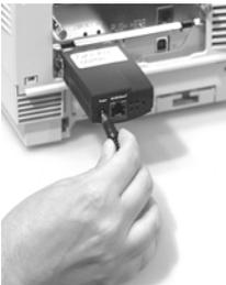
5. Attach the 10/100Base-T UTP cable to the receptacle on the back of the OkiLAN 6020e.
