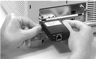
4. Plug the power adapter wire into the power jack on the OkiLAN 6020e. Then plug the power adapter into a 120 VAC wall outlet.
