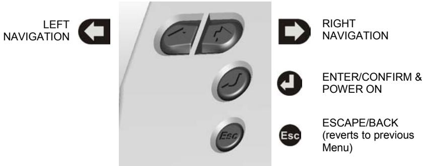
To use the OM-SQ2020/2040 control panel press
