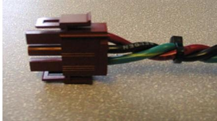
**Note:** If you are not using a Nortel-supplied PDU, have a qualified electrician connect the cable appropriately to your DC power plant. The 1002rp uses a negative 48 V power supply, therefore the red cable is negative (-48 V) and the black cable is the ground (GND).
