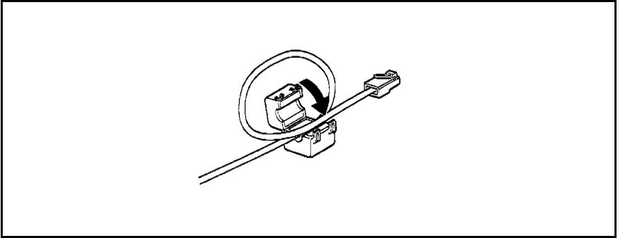
The ferrites are secured to the appropriate cable with plastic enclosure clips. Ty wraps are added to the cable loop.
