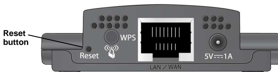
**Figure 6. The Reset button restores factory settings**
