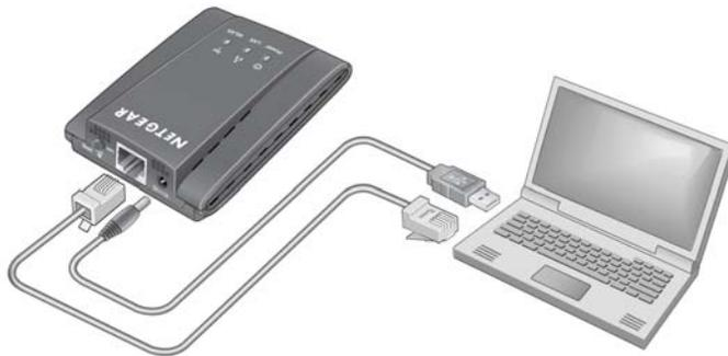
Figure 5. Connecting the Internet adapter to a laptop
