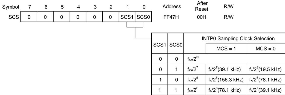
**Caution**  $f_{xx}/2^N$  is a clock to be supplied to the CPU and  $f_{xx}/2^5$ ,  $f_{xx}/2^6$  and  $f_{xx}/2^7$  are clocks to be supplied to the peripheral hardware.  $f_{xx}/2^N$  stops in the HALT mode.
