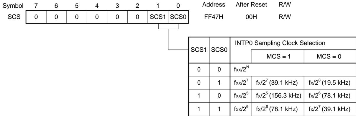
**Caution**  $f_{xx}/2^N$  is the clock supplied to the CPU, and  $f_{xx}/2^5$ ,  $f_{xx}/2^6$ , and  $f_{xx}/2^7$  are clocks supplied to peripheral hardware.  $f_{xx}/2^N$  is stopped in HALT mode.
