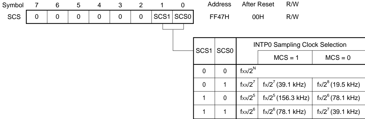
Figure 8-9. Sampling Clock Select Register Format
