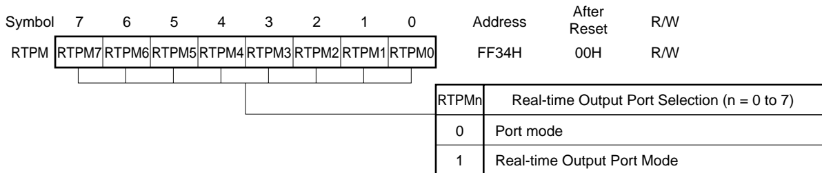
Figure 20-4. Real-time Output Port Mode Register Format
