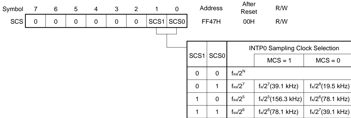
Figure 21-7. Sampling Clock Select Register Format
