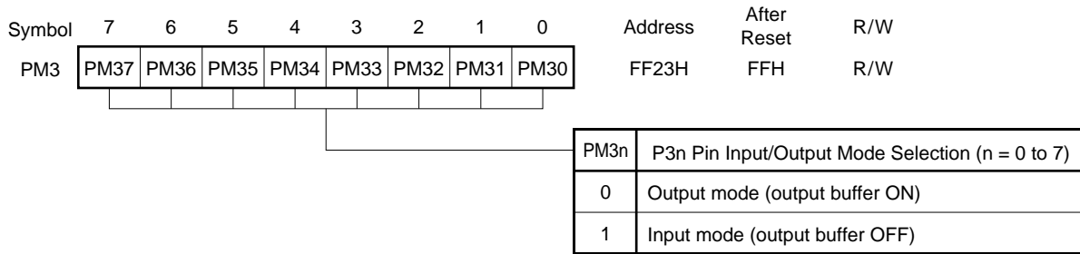
Figure 12-4. Port Mode Register 3 Format
