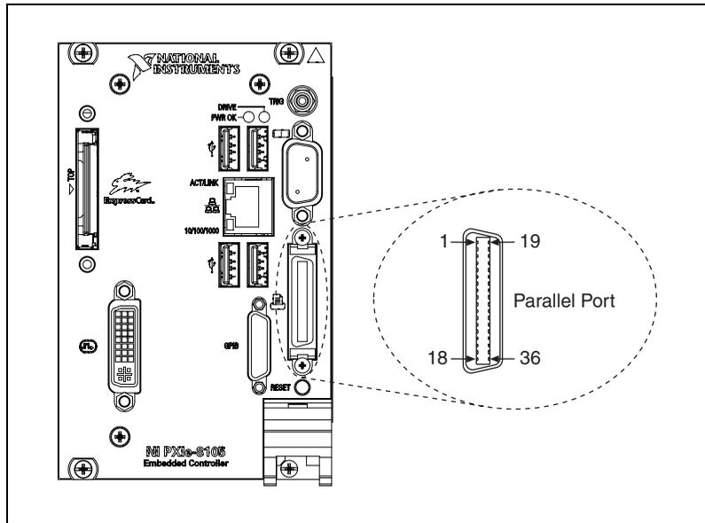
**Figure 3-5.** Parallel Port Connector Location and Pinout
