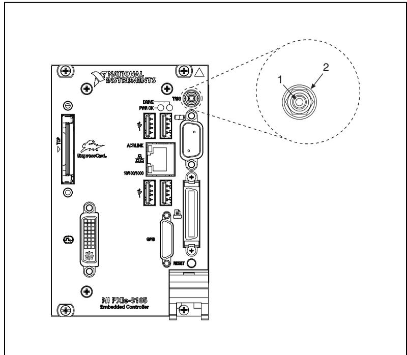
**Figure 3-7.** TRG Connector Location and Pinout
