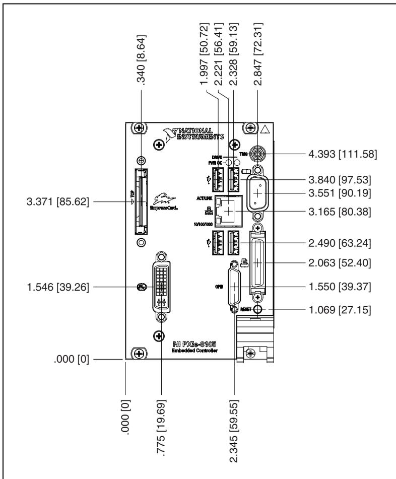
**Figure 3-1.** NI PXIe-8105 Front Panel Layout and Dimensions
