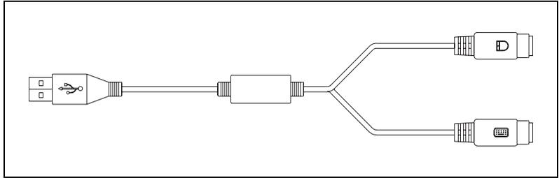
**Figure 4-1.** Y-Splitter Cable
