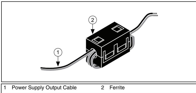
**Figure 5.** Closed Ferrite on the Power Supply Cable
