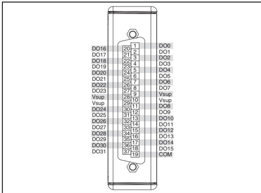
**Figure 1.** NI 9476 Pin Assignments
