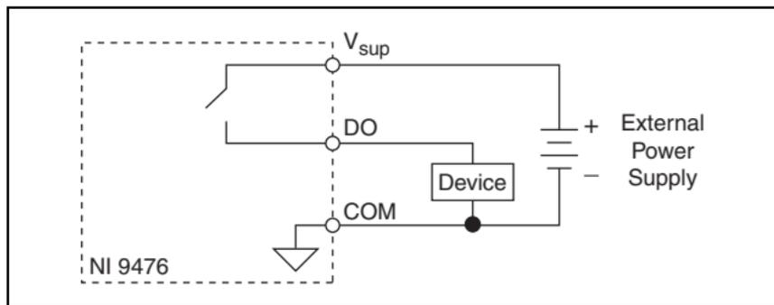
**Figure 2.** Connecting a Device to the NI 9476
