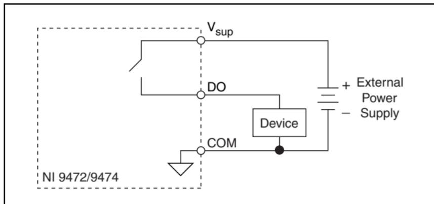
**Figure 3.** Connecting a Device to the NI 9472/9474
