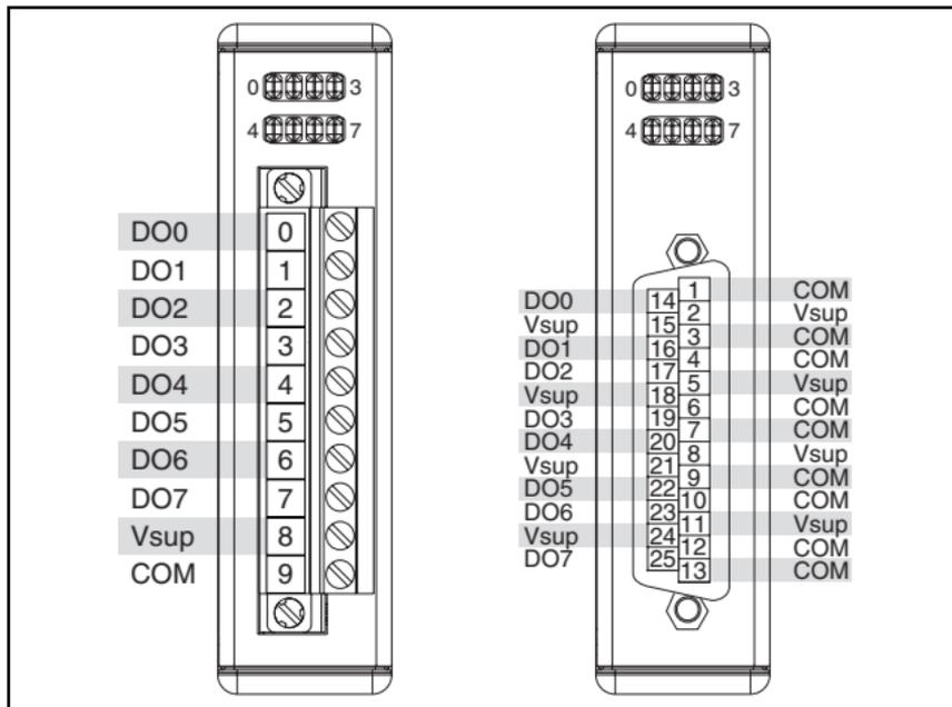
**Figure 2.** NI 9472/9474 Terminal and Pin Assignments
