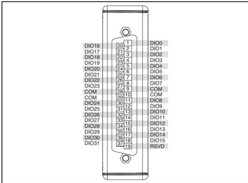
**Figure 1.** NI 9403 Pin Assignments
