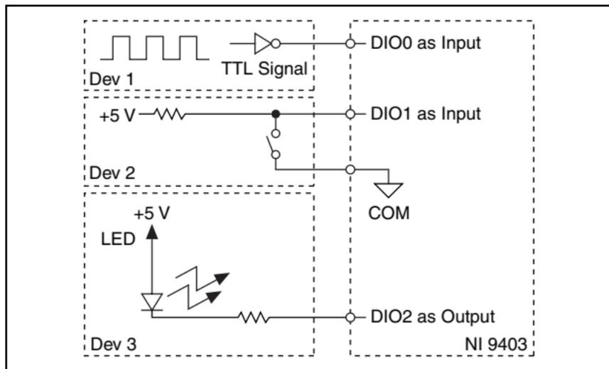
**Figure 2.** Connecting Digital Devices to the NI 9403
