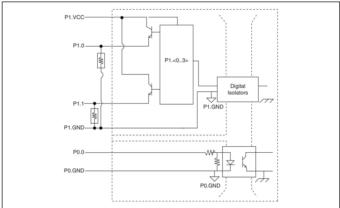
**Figure 8-5.** NI 6232 Digital I/O Connections (DO Source)
