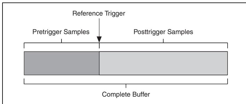
**Figure 4-14.** Reference Trigger Final Buffer
