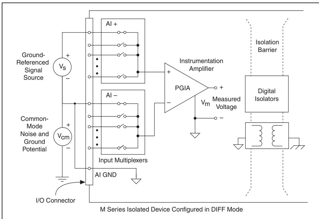
**Figure 4-4.** Differential Connections for Ground-Referenced Signal Sources
