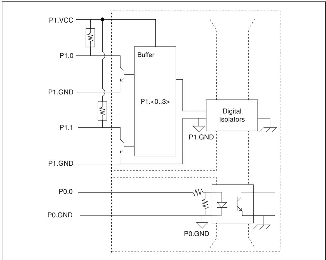
**Figure 6-2.** NI 6233 Digital I/O Connections (DO Sink)
