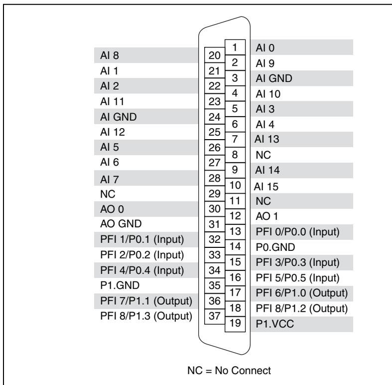
Figure A-2. NI 6233 Pinout
