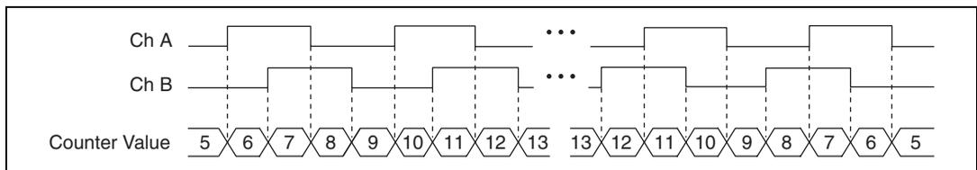
Figure 7-17. X4 Encoding
