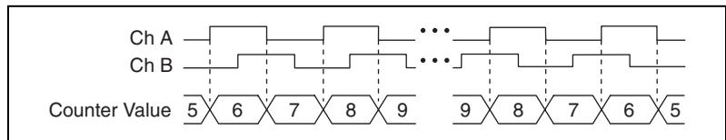
Figure 7-16. X2 Encoding
