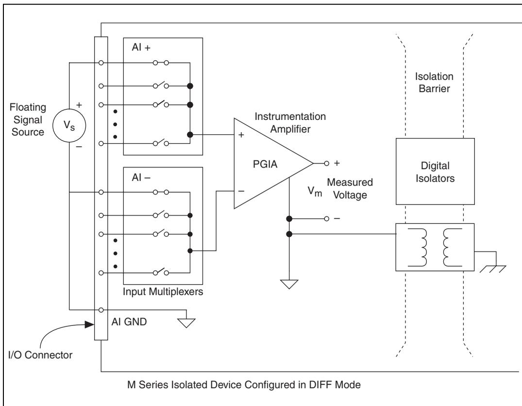
**Figure 4-5.** Differential Connections for Floating Signal Sources
