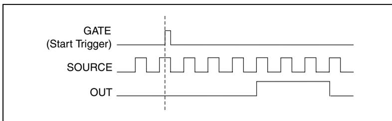
**Figure 7-23.** Single Pulse Generation with Start Trigger
