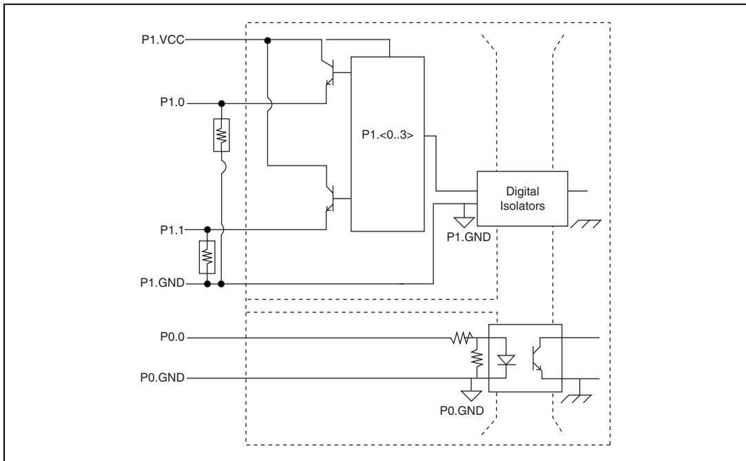
**Figure 6-1.** NI 6232 Digital I/O Connections (DO Source)
