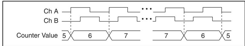
Figure 7-15. X1 Encoding
