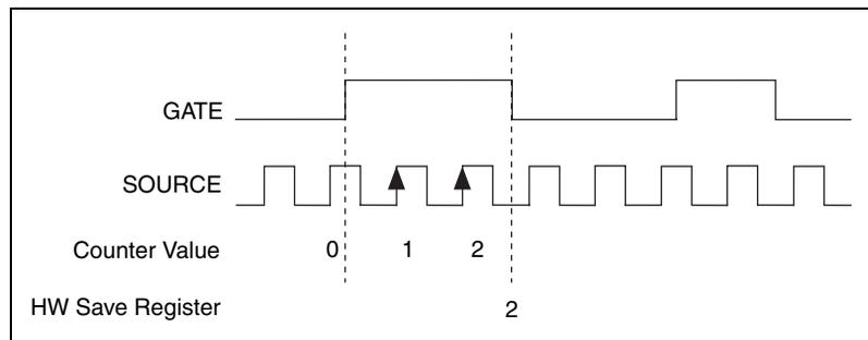
**Figure 7-6.** Single Pulse-Width Measurement
