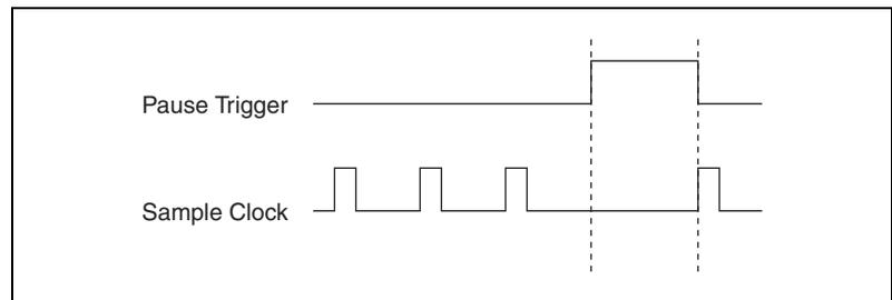
**Figure 5-4.** ao/PauseTrigger with the Onboard Clock Source
