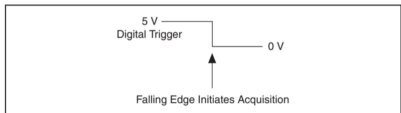
**Figure 12-1.** Falling-Edge Trigger
