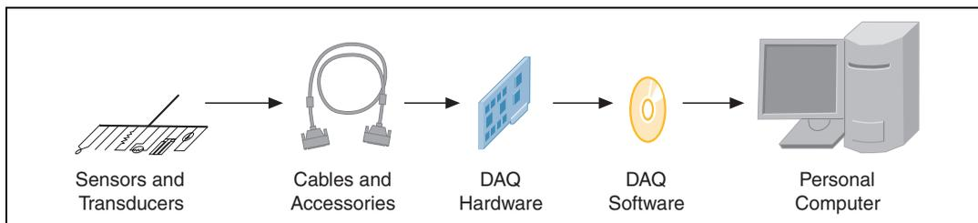
**Figure 2-1.** Components of a Typical DAQ System
